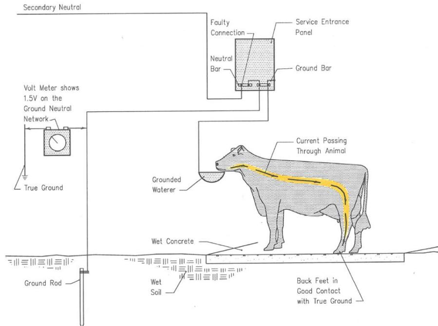
Figure 1 One Example of Stray Voltage<sup>2</sup>
